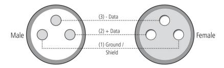
Resistance 120 ohm // 1/4 w between pin 2 (DMX-) and pin 3 (DMX+) oft he last fixture.
